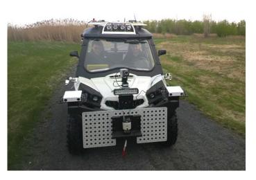
Figure 3–11: The participant, sitting in the SL-Commander's passenger seat, collaborated with our adaptive boundary tracking agent during the APEX interactive driving field demonstrations. А human driver was also and provided present redundant safety duties by maintaining access to the vehicle's brake pedal and emergency stop buttons.
