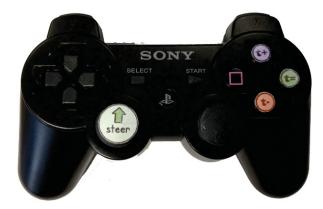
Figure 4–8: Gamepad interface for the real-time trust dynamics study included additional labels annotating the analog stick for manual interventions use (steer), as well as buttons for issuing trust change critiques (t+, t=, t-). intervention state  $i \in \{0, 1\}$  at that time. We also noted frames in proximity to a change-over between boundary targets, corresponding to external intervention causes  $e \in \{0, 1\}$ .
