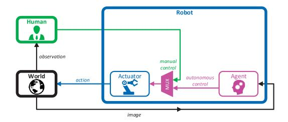
Figure 1–2: In a supervisor-worker team, the autonomous *agent* onboard the mobile robot senses the state of the world (e.g. using a camera) and generates control commands to the vehicle's low-level *actuator*. Meanwhile, a *human* supervises the robot's task performance by observing its behaviors, and can also issue intervening control signals to the robot's actuator. A command multiplexer (MUX) ensures that the supervisor's interventions always supersede the agent's commands.
