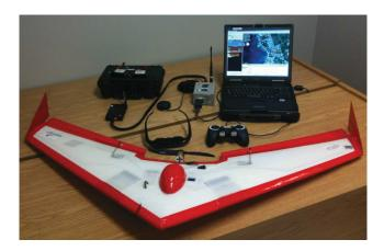
Figure 2–2: The Unicorn is a commercial fixed-wing Unmanned Aerial Vehicle with an on-board autopilot microprocessor and gimbal-mounted camera.
