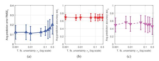
Figure 5–8: Means and standard deviations (as error bars) of OPTIMo's prediction performances as functions of the trust feedback uncertainty parameter  $\sigma_f$  (with W = 3 s, B = 300 bins,  $\sigma_t = 0.005$ ).
