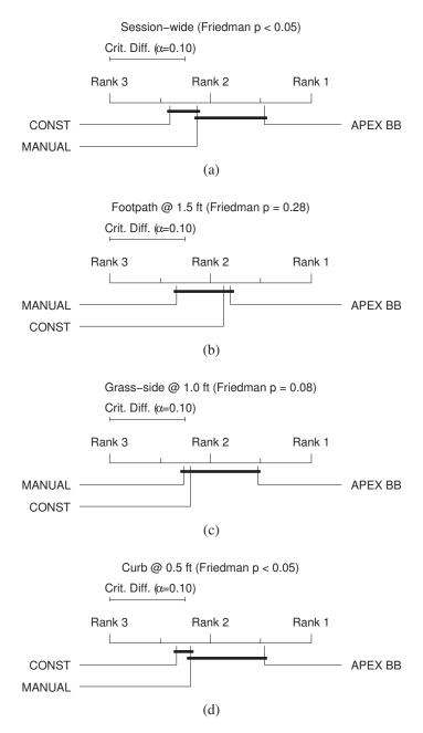
Figure 3-9: Critical difference plots from the campus patrol field trial indicated that the APEX ΒB adaptive agent consistently contributed to the greatest overall efficiency team in comparison to both the non-adaptive CONST agent and the baseline MANUAL teleoperated configuration. Post hoc Nemenyi analysis revealed the lack of significant differences the presence of (i.e. thick horizontal lines straddling multiple agents) among these orderings.
