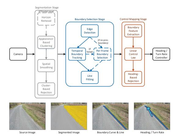
Figure A–2: Our boundary tracking pipeline consist of segmenting terrain patches in each camera frame, selecting a target boundary to track across frames, and mapping boundary data into steering commands; dashed blocks depict conditional steps.
