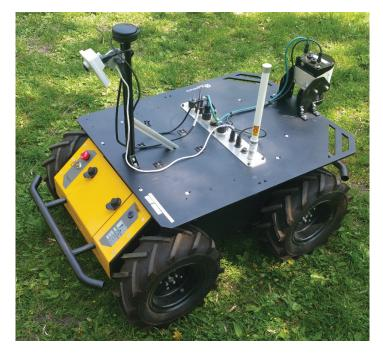
Figure 2–4: The Husky is a commerciallyavailable wheeled robot for outdoor research. This robot is equipped with assorted sensors, including a GPS receiver, an IMU, a laser range-finder, and a camera with adjustable pitch and roll.
