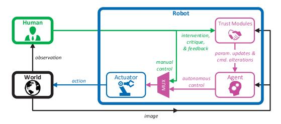
Figure 1–3: Our trust-seeking robot framework enhances a plain supervisor-worker team with *trust modules* serving diverse purposes. These modules update the agent's parameters to adapt to occasional human interventions, infer the supervisor's level of trust in the robot based on reactions and feedback, and help the robot agent regain lost trust by altering its behaviors.
