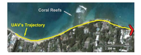
Figure A–5: Our fixed-wing UAV (red icon) executed multiple flights over a 1km target stretch of tropical shoreline during our coastline tracking field trial.
