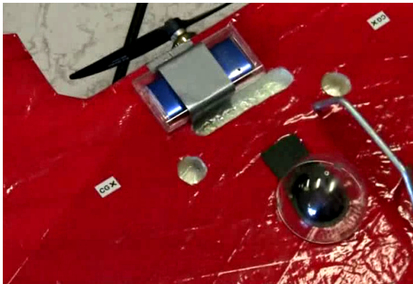
Figure A–3: The Unicorn UAV’s integrated camera (black unit) is attached to a gimbal and is protected by a transparent plastic hull. We also secured an iPod nano to the UAV’s underbelly to record high-resolution flight footage that are devoid of analog transmission artifacts.
