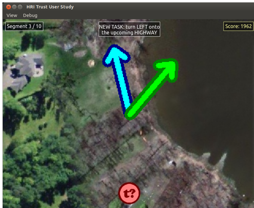
Figure 4–7: The display interface for the real-time trust dynamics study mostly resembled the camera view from the previous event-centric trust changes study. This view depicted the detected boundary (blue line), steering commands from the robot agent and human (as blue/green arrows), as well as text overlays denoting the session ID, the current task goal, and the tracking performance score.
