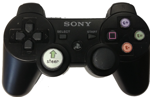
Figure 4–8: Gamepad interface for the real-time trust dynamics study included additional labels annotating the analog stick for manual interventions use ( steer ), as well as buttons for issuing trust change critiques ( t+ , t= , t- ).
