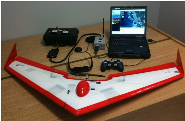
Figure 2–2: The Unicorn is a commercial fixed-wing Unmanned Aerial Vehicle with an on-board autopilot microprocessor and gimbal-mounted camera.
