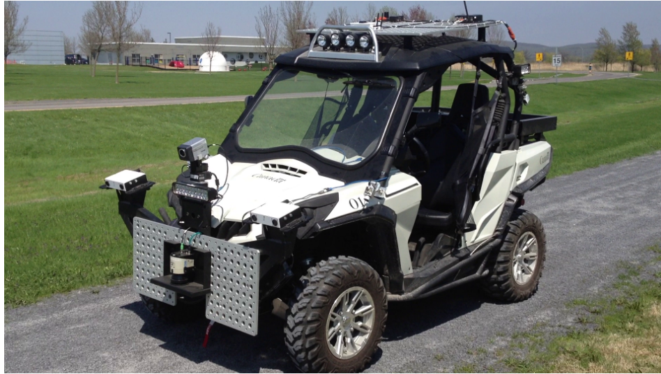
Figure 2–5: The SL-Commander ATV is a custom research platform featuring a programmable drive-by-wire control interface and houses many sensors including cameras, a laser range-finder, a GPS unit, and an IMU.
