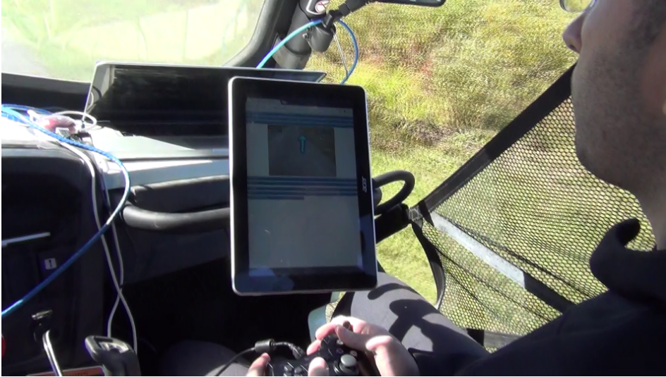
Figure 6–9: During the TACTiC field trial extension, the participant sat in the SL-Commander’s passenger seat and interacted with boundary tracking agents using the same gamepad interface from the TACTiC user study, while a tablet below the windshield displayed the agent’s overlaid camera visualizations and post-session trust feedback questionnaire.
