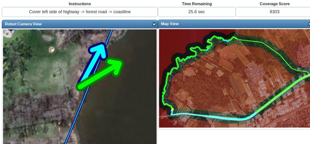
Figure 3–1: The APEX aerial coverage user study features a two-pane display interface. The left view shows frames from the simulated drone’s downward-facing camera, overlaid with the detected boundary (blue line) and the agent’s/supervisor’s angular rate steering commands (blue/green arrows). The right map view depicts covered/missed portions of the flight course (green/cyan regions), the robot’s current position (yellow square near the lower-left corner), and out-of-bound areas (red-tinted regions).
