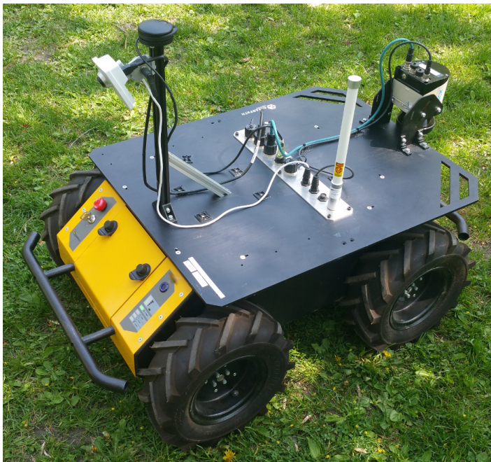
Figure 2–4: The Husky is a commercially-available wheeled robot for outdoor research. This robot is equipped with assorted sensors, including a GPS receiver, an IMU, a laser range-finder, and a camera with adjustable pitch and roll.
