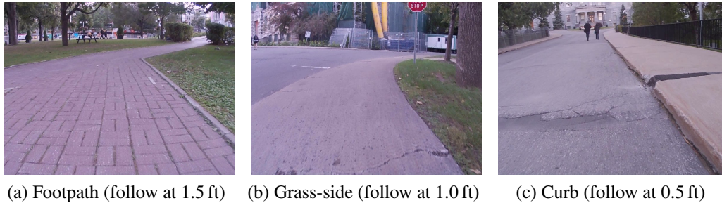
Figure 3–7: The test course for the APEX campus patrol field trial consisted of moving alongside a sequence of terrain boundaries with visually-defined transition points. Boundary targets had varied visual appearances and included a footpath segment (a), a grass-side sidewalk section (b), and a road-side curb (c).
