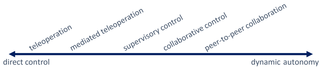
Figure 2–1: Goodrich and Shultz’s classification of levels of autonomy with emphasis on human interaction (replicated from [38]).
